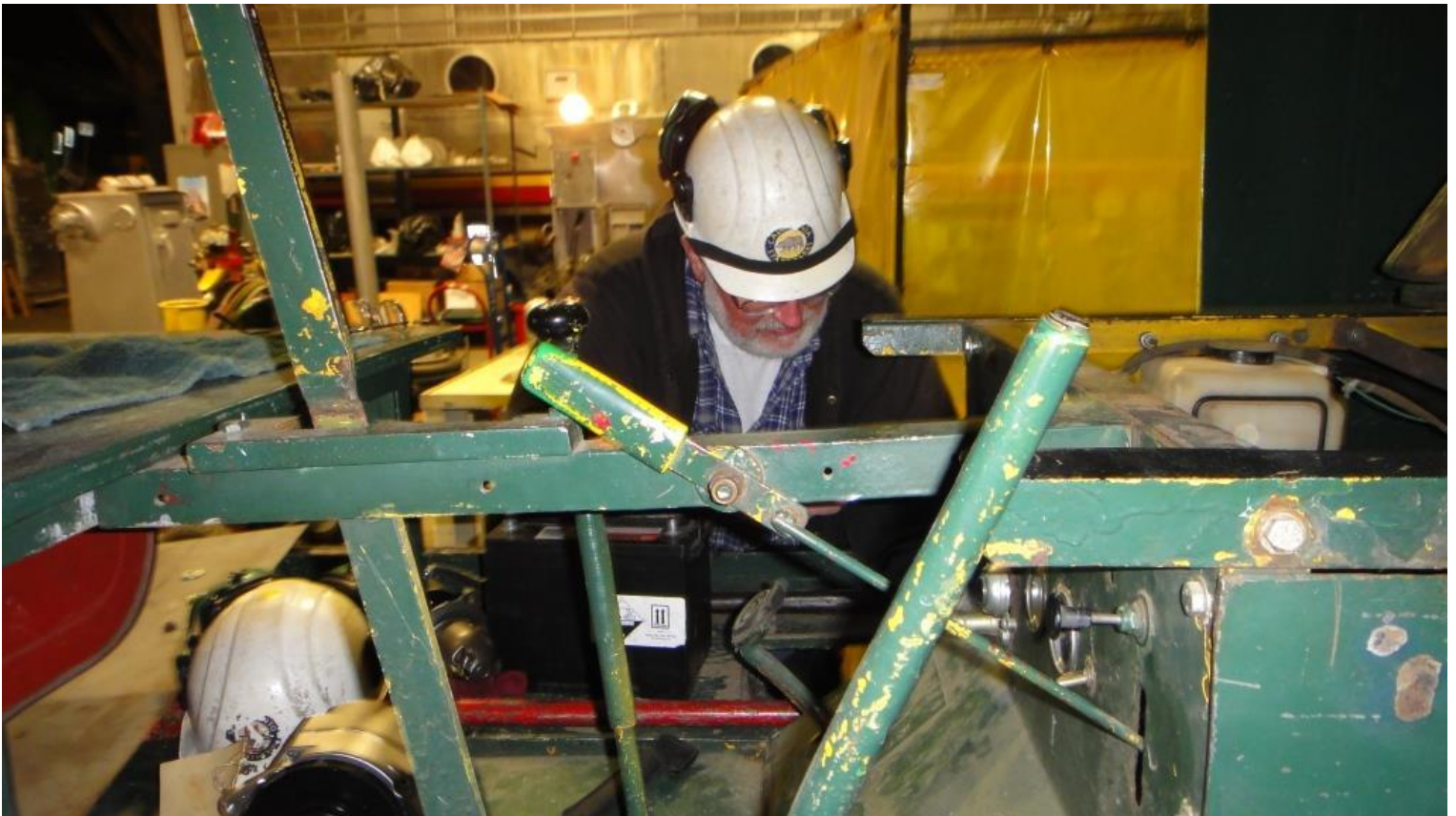
Frank connecting the new starter-motor on the A-5 motorcar
