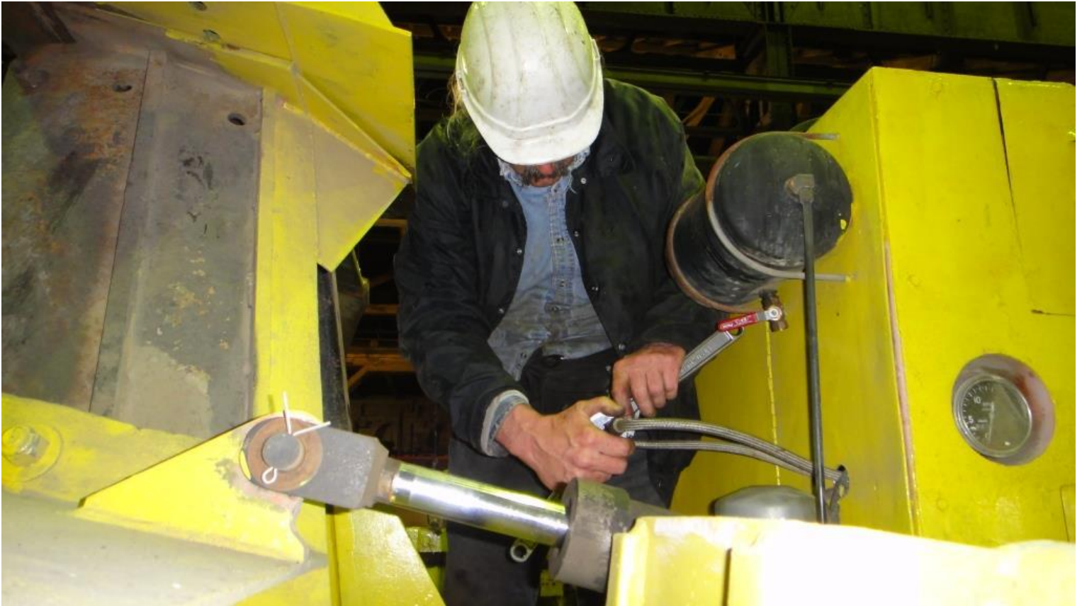
Fred bypassing the air-dryer on the regulator as a trouble-shooting measure
